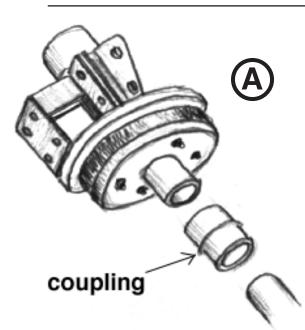
The well-seal slips on to the 5-foot top-section (with the weep-hole label) directly below the steel hanging bracket (**see illustration "A**").
