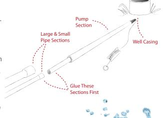
CRITICAL-Before gluing anything, read, understand and follow the instructions for your PVC cleaning and priming solutions, and the adhesive. Glue joints are critical, and are your responsibility. Both the male and female parts of each joint must be cleaned, primed and glued. Short cuts could result in pump failure or dropping your pump into the well. Also, the factory-knots on the drop-line are for positioning only, and must be checked and re-tied adequately.
