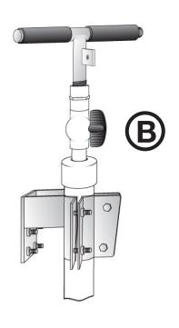
Caution--Be very careful NOT to drop the pump shaft into the pump. Retrieval is difficult. As a precaution, lift the handle and tape a cross piece of pipe to the <sup>3</sup>/<sub>4</sub>" shaft to keep it from dropping as you work.
