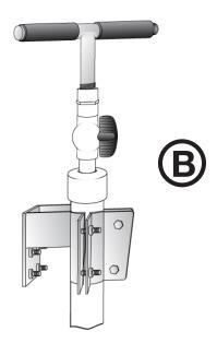
Caution--Be very careful NOT to drop the pump shaft into the pump. Retrieval is difficult. As a precaution, lift the handle and tape a cross piece of pipe to the ¾" shaft to keep it from dropping as you work.
