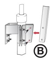
Note: Your PowerJak comes from the factory with the drop-link bolted in the center position on your lever handle. Depending on the system mounting height, and the height of the operator, the bolted location may be adjusted to minimize pumping friction against the debris cap. If
